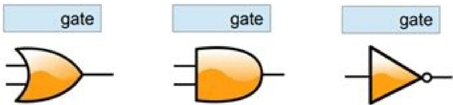
This gate takes two inputs and gives an output if either one input or the other input or both inputs are true
